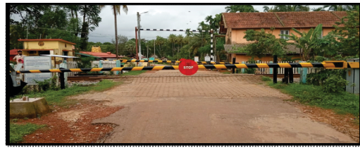
MLCG with Booms Electrical operation & boom locking
